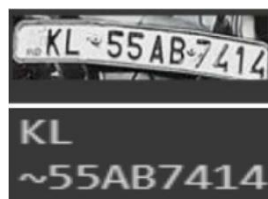
Fig.9.Easy OCR output after number plate recognition
