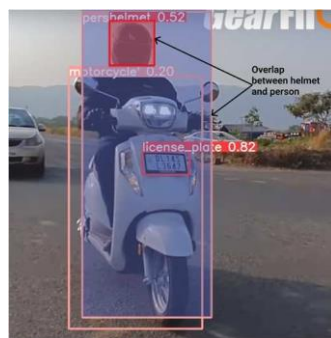
Fig 3.a Checking Overlap between helmet and person class Method1
