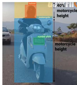
Fig 3.d Checking if the helmet is present 40% above the height of the motorcycle- Method2
