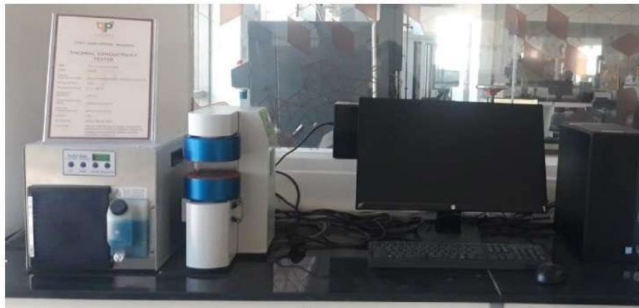
Fig. 2. FOX 50 heat flow meter experimental setup to measure thermal conductivity.
