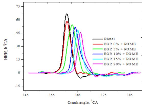
Fig. 9: Effect of EGR, nozzle geometry, IT and CC shape on the heat release rate
