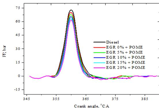
Fig. 8: Effect of EGR, nozzle geometry, IT and CC shape on peak pressure
