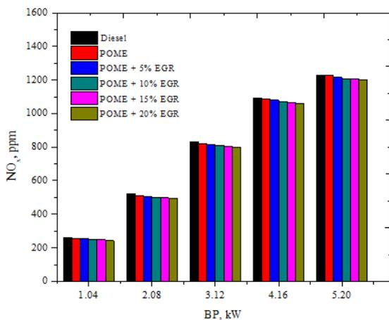
Fig.7: Effect of EGR, nozzle geometry, IT and CC shape on NO<sub>x</sub> emissions
