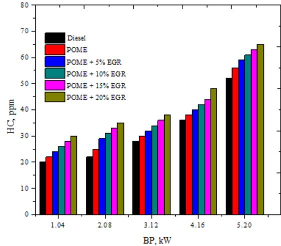
Fig. 5: Effect of EGR, nozzle geometry, IT and CC shape on Unburned Hydrocarbon Emissions
