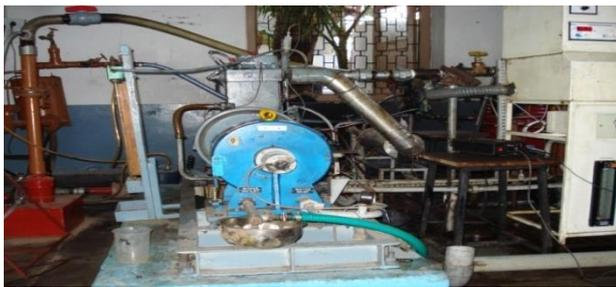
Fig. 1: Experimental setup with EGR arrangement
