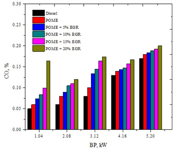
Fig. 6: Effect of EGR, nozzle geometry, IT and CC shape on Carbon monoxide emissions
