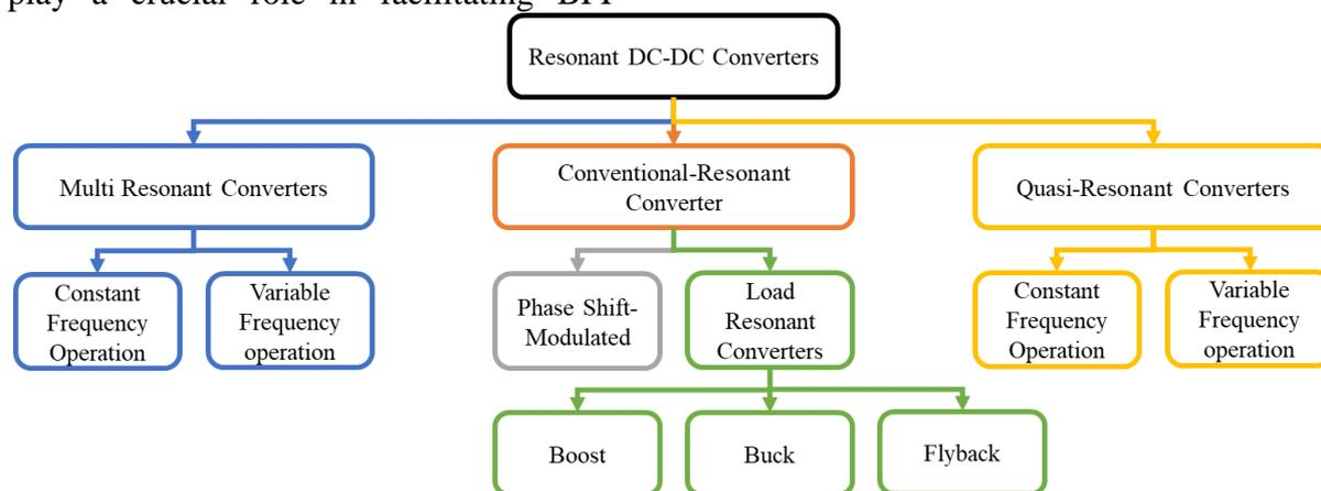
Figure 5. Taxonomy of Resonant DC-DC Converters
