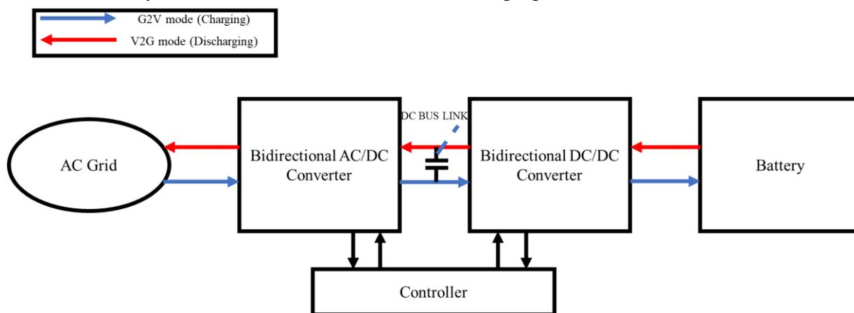
Figure 6. EV bidirectional charger topology [23].
