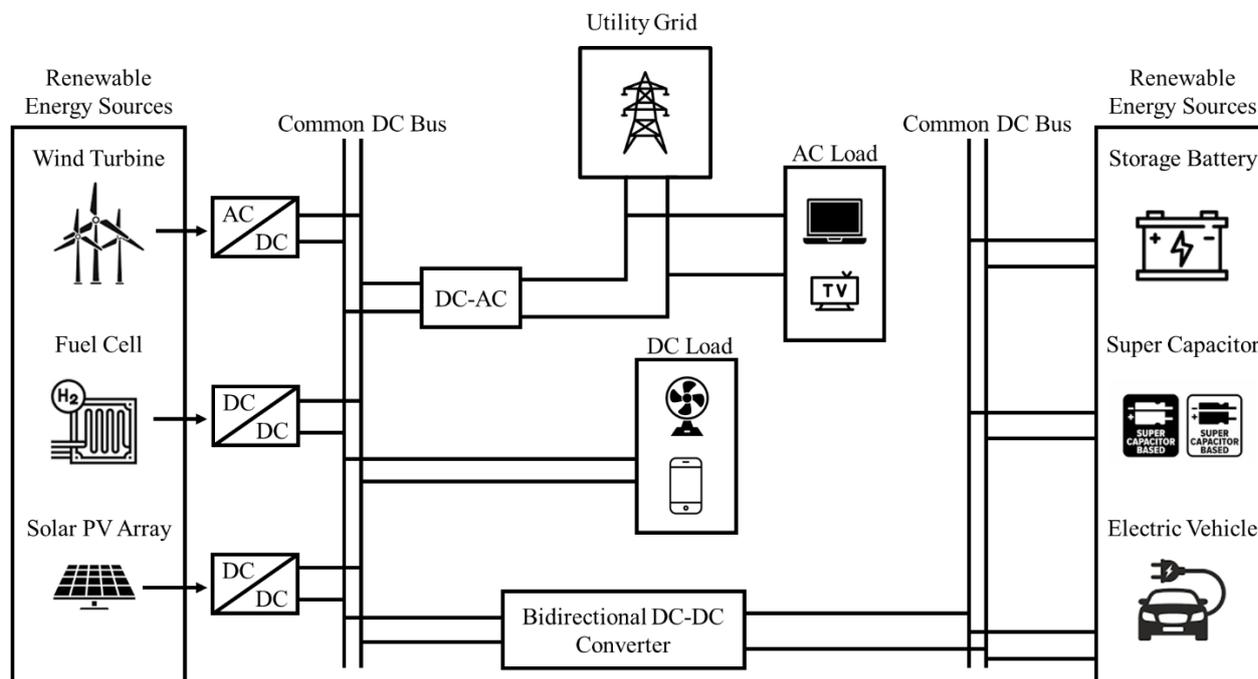
Figure 1. Enhancing Renewable Energy Systems with Power Electronic Converters. [11]
