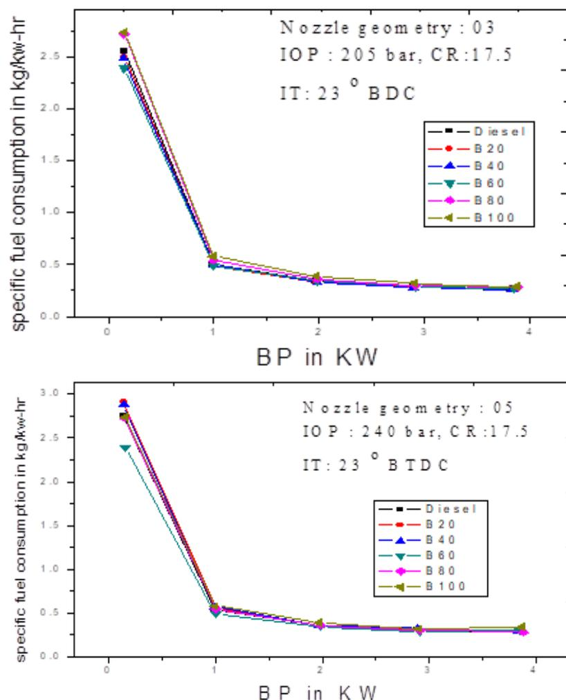
**Fig.3.** Variation of SFC with BP for baseline and modified nozzle geometries
