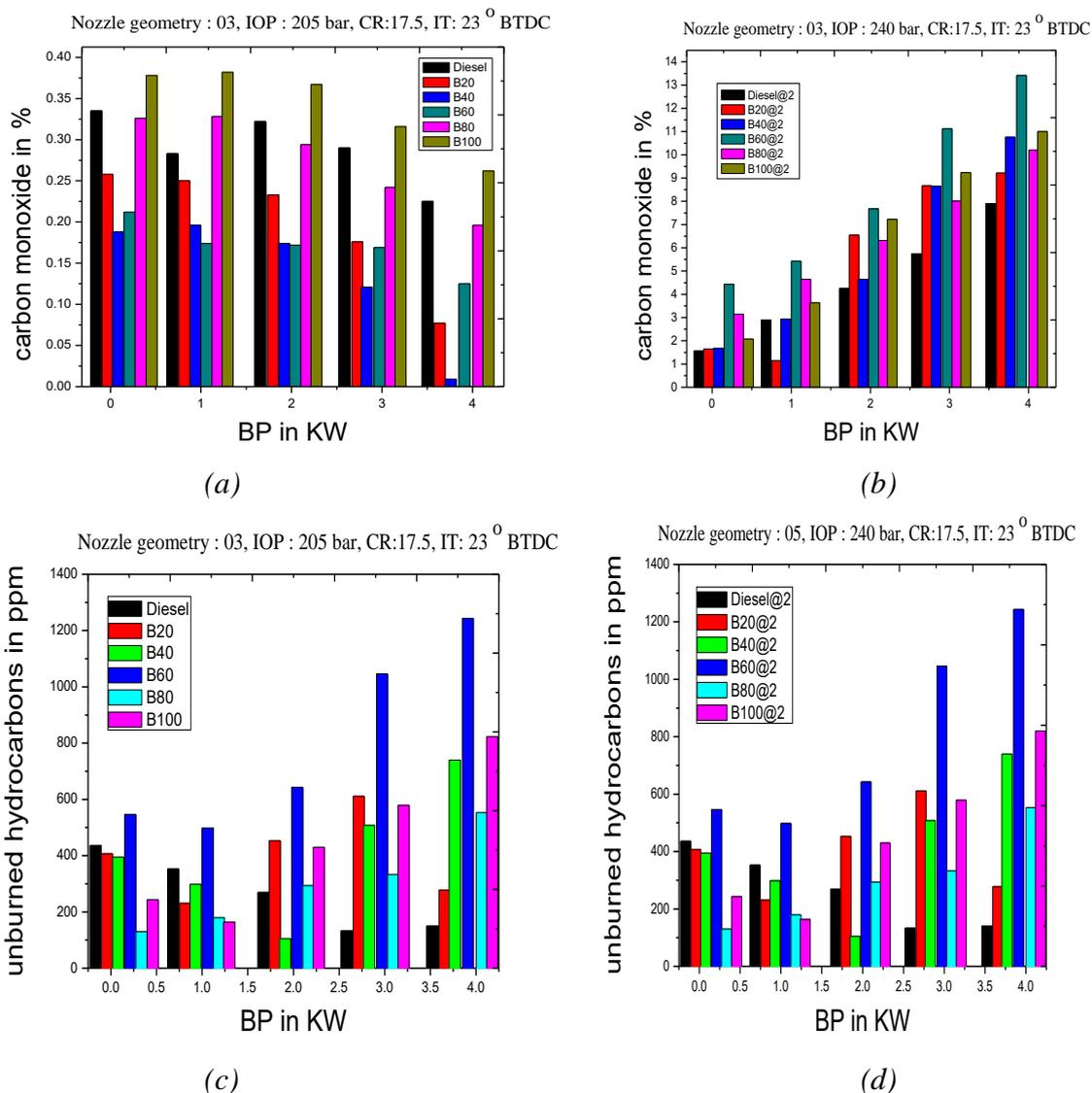
Fig.5. Variation of CO and UBHC emissions with BP for baseline and modified nozzle geometries
