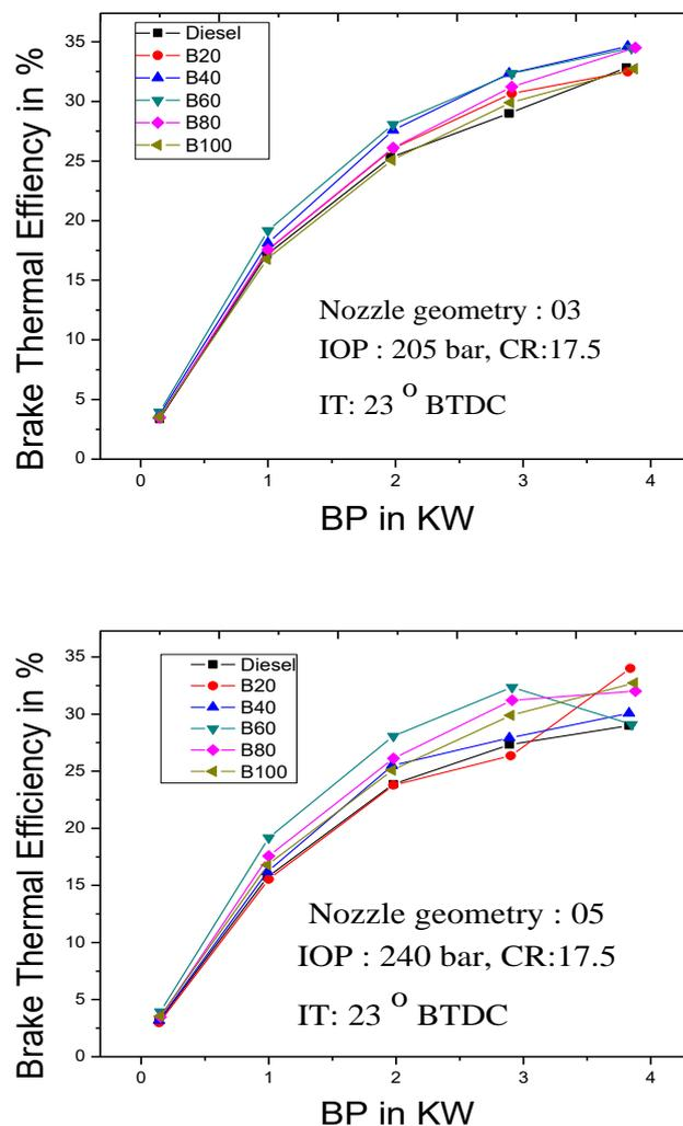
**Fig.4.** Variation of BTE with BP for baseline and modified nozzle geometries
