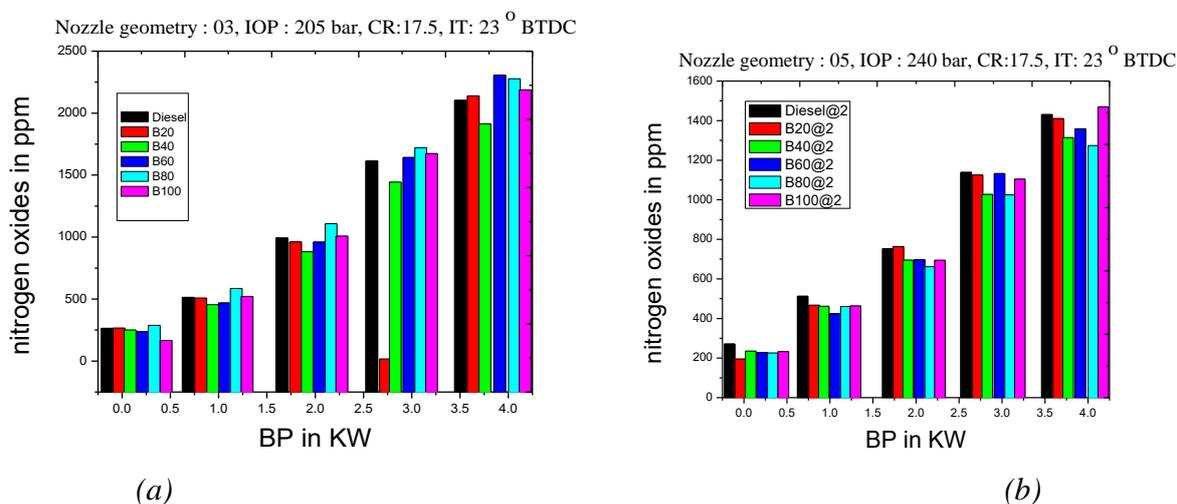
Fig.6. Variation of NO<sub>x</sub> emissions with BP for baseline and modified nozzle geometries
