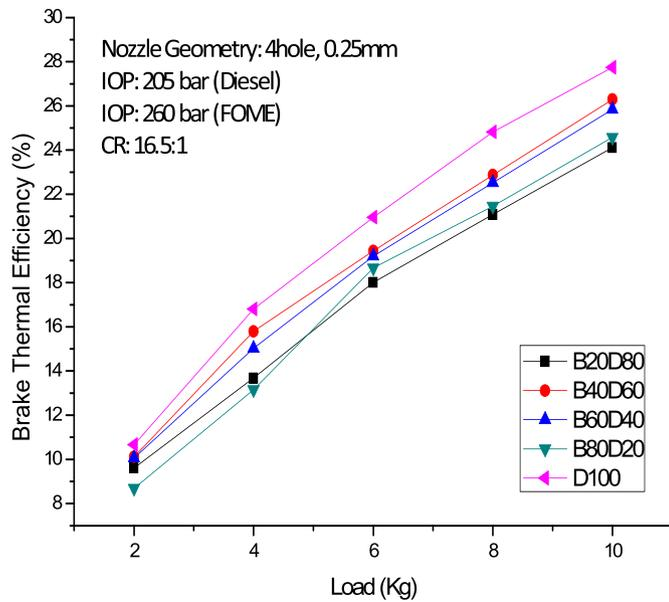
Fig. 11. Variation of brake thermal efficiency with load.
