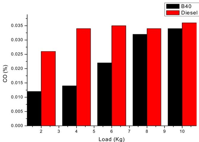
Fig. 31. Variation of carbon monoxide with load.
