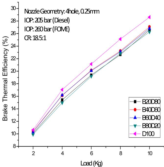
Fig. 27. Variation of brake thermal efficiency with load.
