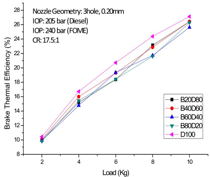
Fig. 13. Variation of brake thermal efficiency with load.
