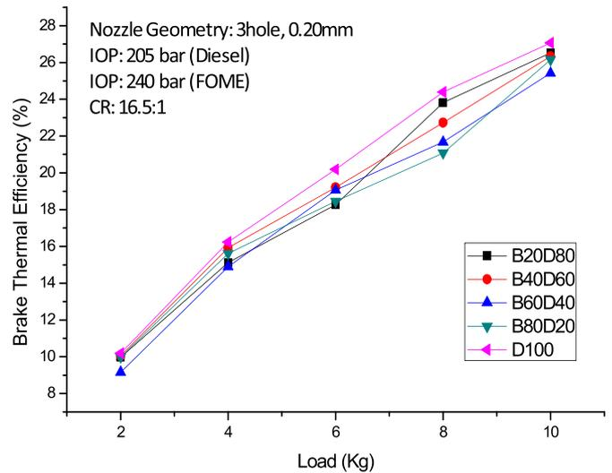
Fig. 5. Variation of brake thermal efficiency with load.
