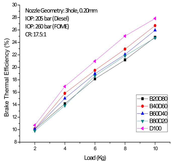
Fig. 17. Variation of brake thermal efficiency with load.
