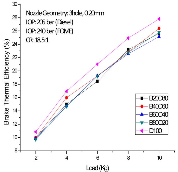
Fig. 21. Variation of brake thermal efficiency with load.
