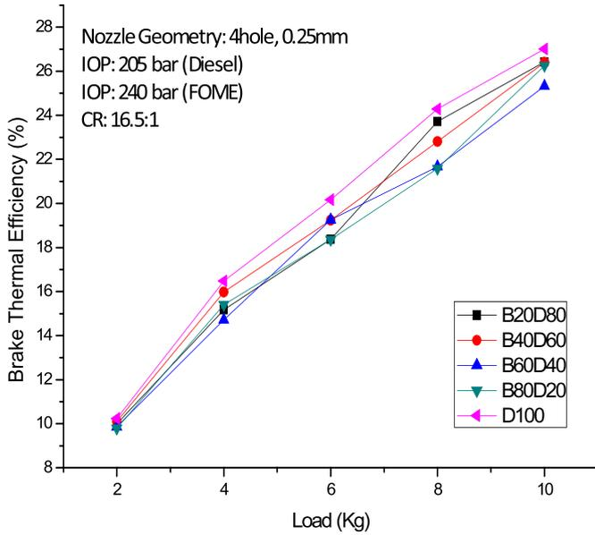
Fig. 7. Variation of brake thermal efficiency with load.
