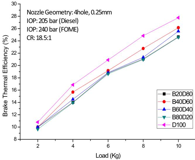
Fig. 23. Variation of brake thermal efficiency with load.
