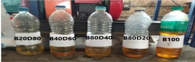
**Fig. 1.** Blends of Biodiesel and diesel.
