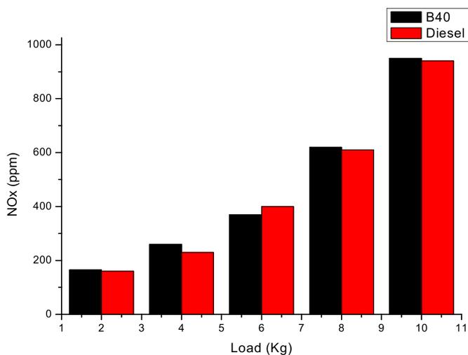
Fig. 33. Variation oxides of nitrogen with load.
