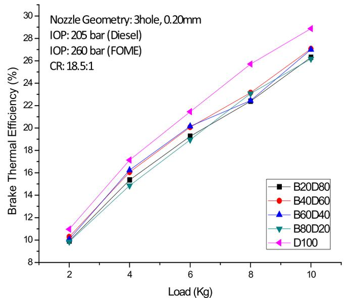
Fig. 25. Variation of brake thermal efficiency with load.
