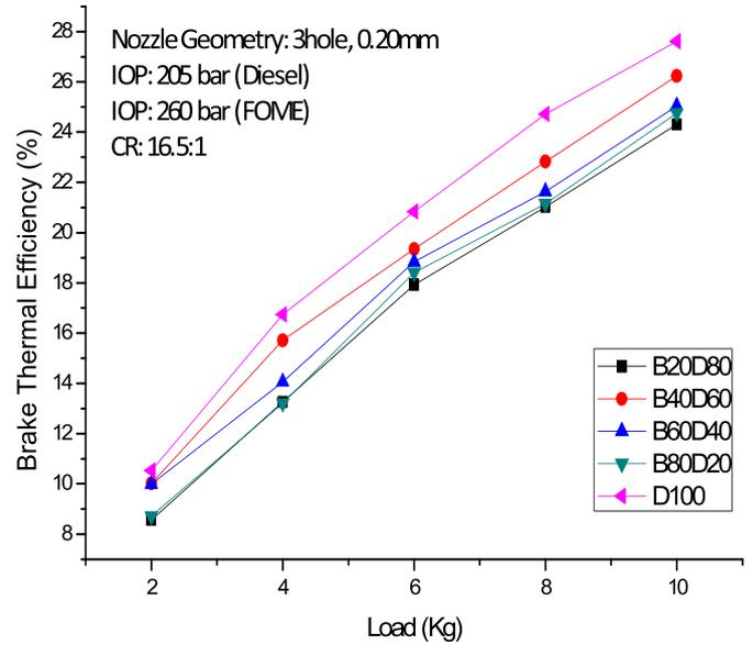
Fig. 9. Variation of brake thermal efficiency with load.
