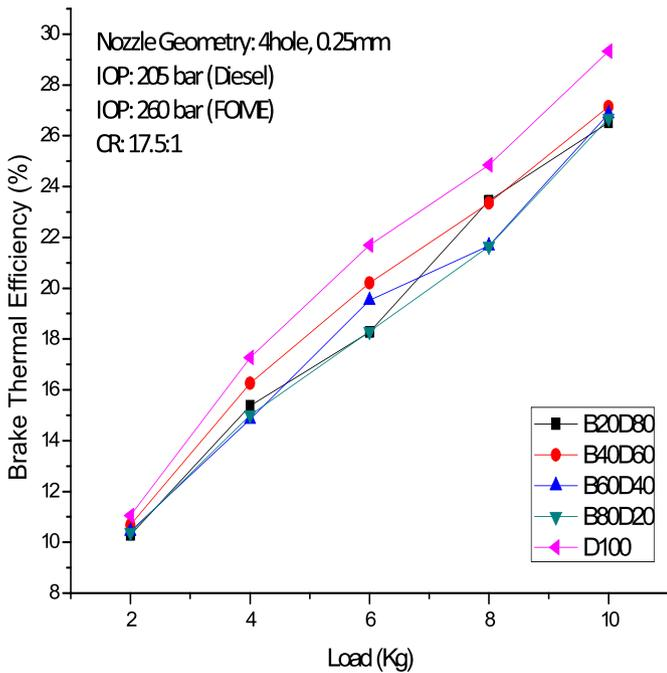
Fig. 19. Variation of brake thermal efficiency with load.
