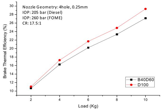
Fig. 29. Variation of brake thermal efficiency with load.
