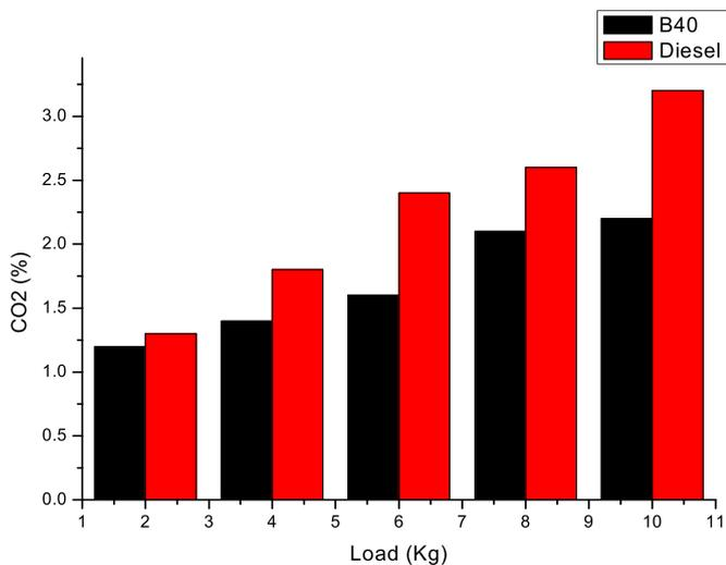
Fig. 32. Variation of carbon dioxide with load.
