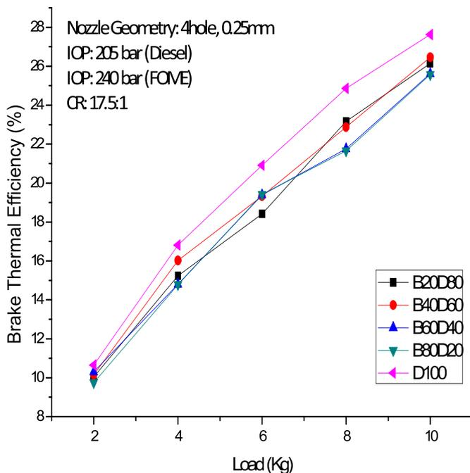
Fig. 15. Variation of brake thermal efficiency with load.
