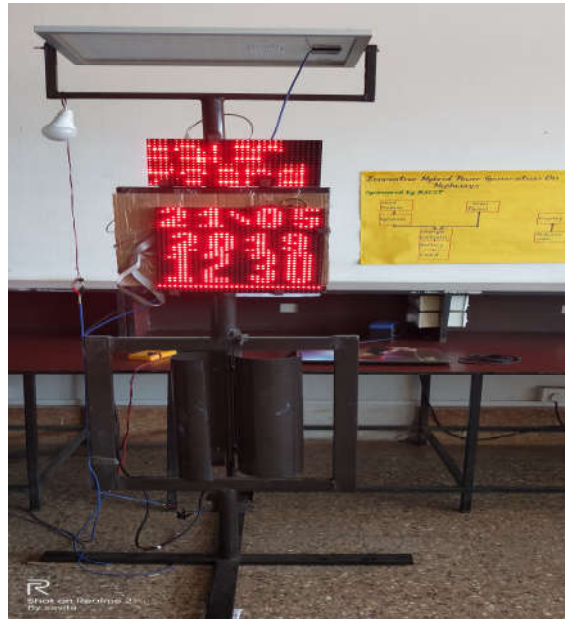
Fig. 4 Hardware Connection Setup for Innovative Hybrid Power Generation On Highways.
