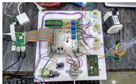
The implementation of this project mainly requires development of the hardware using sensors and raspberry pi model B then programming it to achieve the desired result. When the Linux operating system is installed on the raspberry pi and the peripherals such as monitor, keyboard, mouse, SD card, power supply etc, then it acts as the mini computer system.
