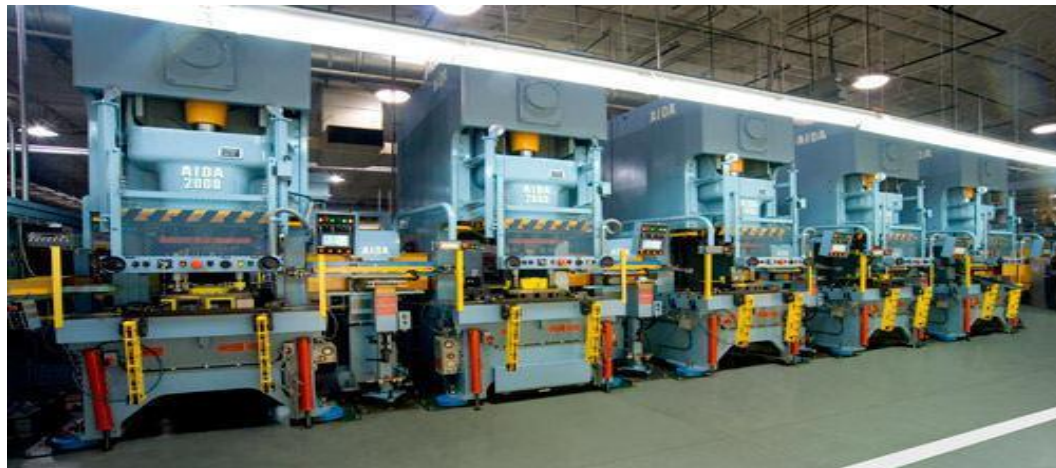
Figure 26 Example of 20 stations Transfer line
