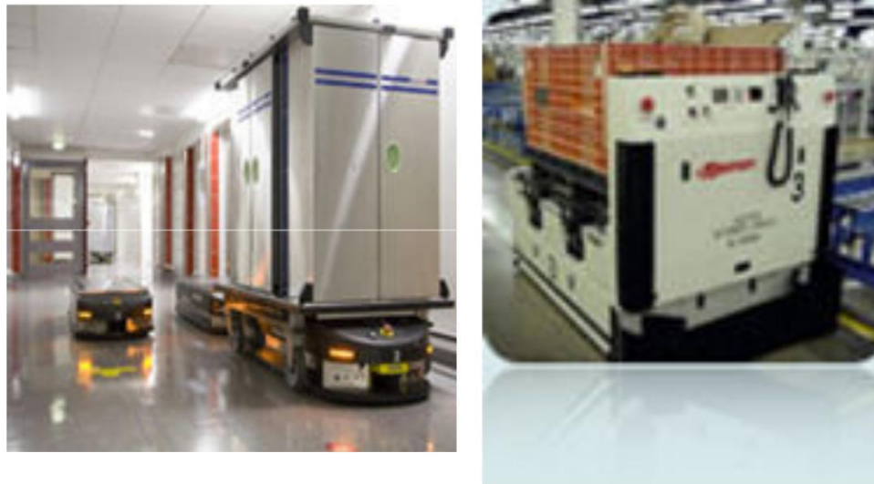
Figure 21 AGV unit load carrier
