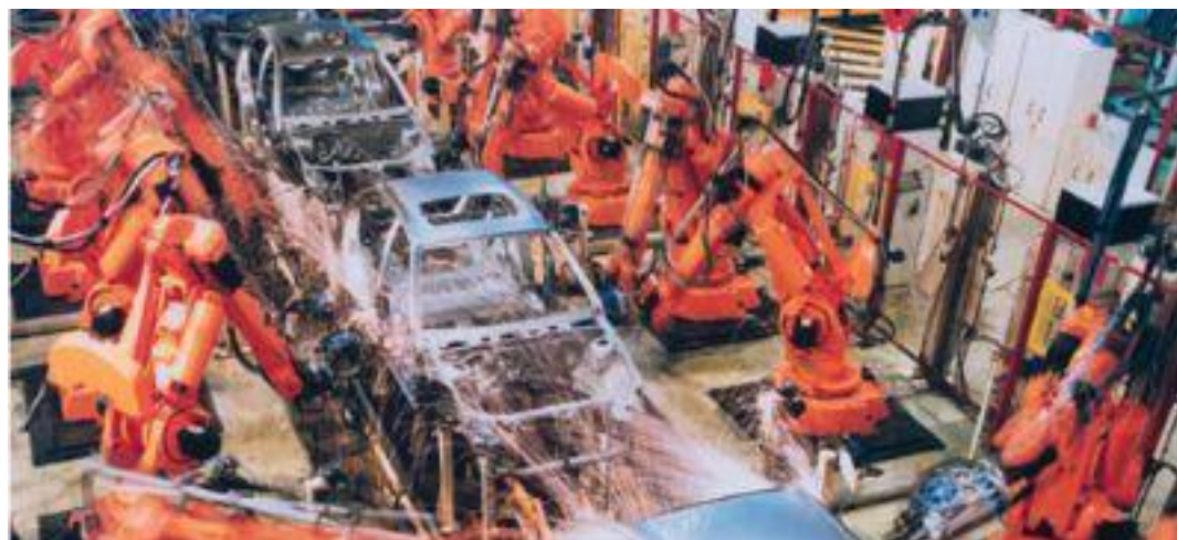
Figure 27 Example of Transfer line
