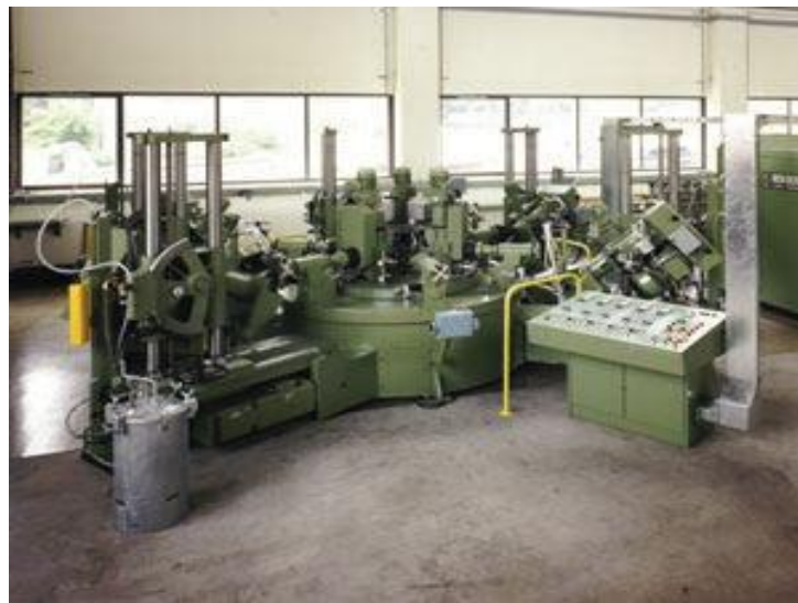
Figure 22 Example of 6 station rotary configuration
