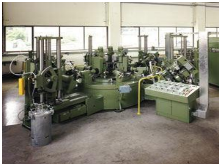
Figure 9 Example of 6 station rotary configuration
