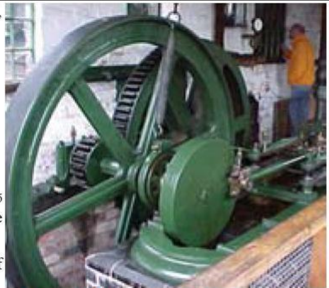
A flywheel stores energy when the supply is in excess and releases energy when energy is in deficit.
