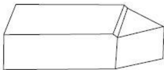
Fig. .4 Solid type of single point cutting tool
