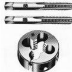
Thread tap and die made of high-speed steel
