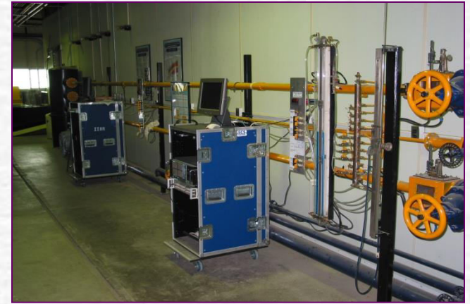
Lab2: Measurement of flow rate, friction factor and velocity profiles in smooth and rough pipes.
