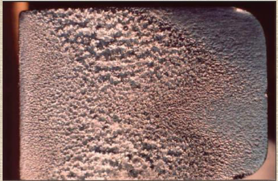
Cavitation damage on a 16-mm by 23-mm aluminum sample tested at 60 m/s for 2.5 h. The sample was located at the cavity collapse region downstream of a cavity generator specifically designed to produce high damage potential.
