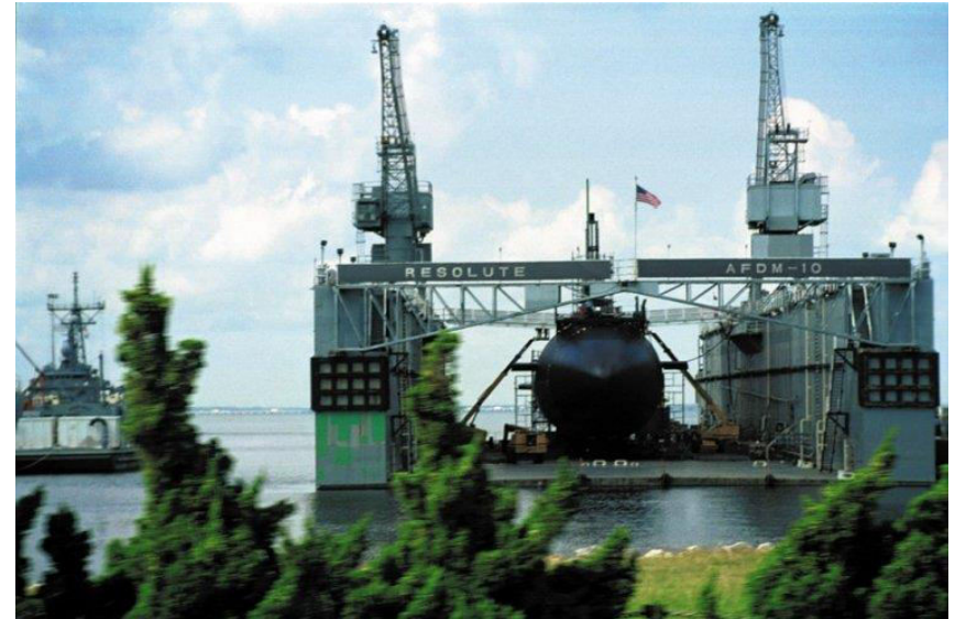
Submarine undergoing repair work on board the AFDM-10
