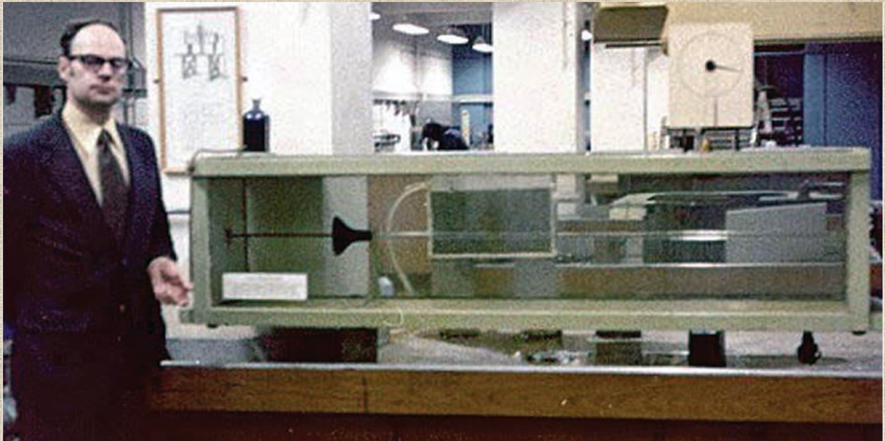
Osborne Reynolds' original apparatus for demonstrating the onset of turbulence in pipes, being operated by John Lienhard at the University of Manchester in 1975.
