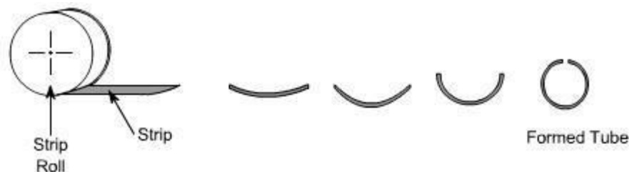
Fig 11.10: Forming of Tube from Strip
