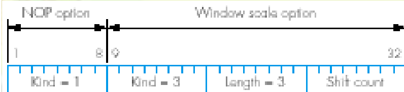
Figure 12.16 Window scale option format.
