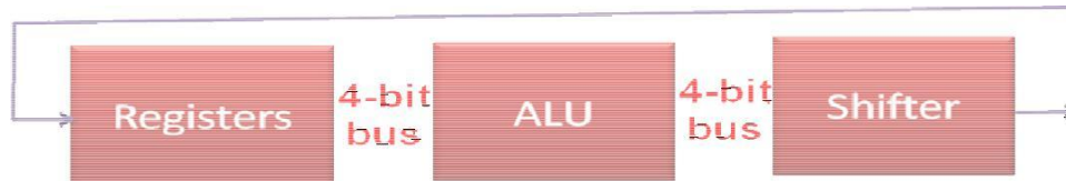
Figure : One bus architecture Sequence:
