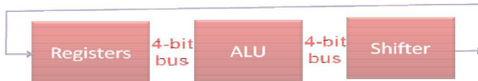
Figure 6.4: One bus architecture
