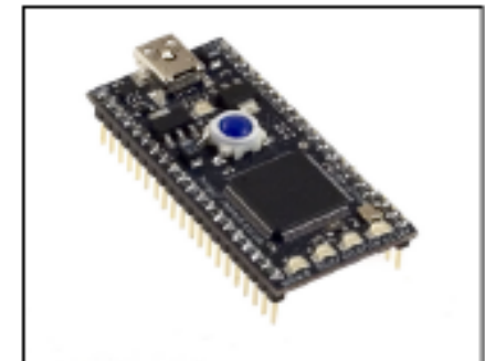
Cortex-M3 MCU in a Prototyping Form-Factor
