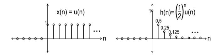
We wish to find the step response s(n) of the system (i.e. the response of the system to the unit step input x(n) = u(n). This is shown below.
