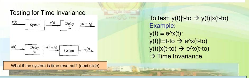
Time-shift in input results in time-shift in output  $\rightarrow$  system always acts the same way (Fix System)
