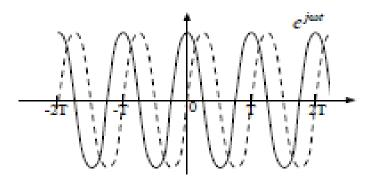
Real sinusoid can be represented as the real part of a complex sinusoid
