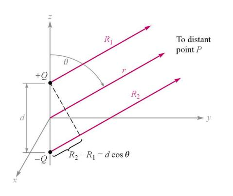
To approximate the potential of a dipole, assume R1 and R2 are parallel since the point P is very distant
