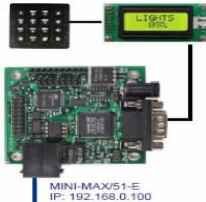
Operator Terminal Station 1
