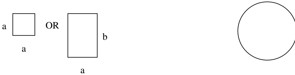
Square or rectangular core with square or rectangular coil Stepped leg (Uses only circular coil)
