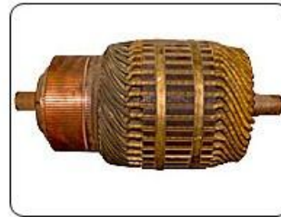
Armature with steel binding wire
