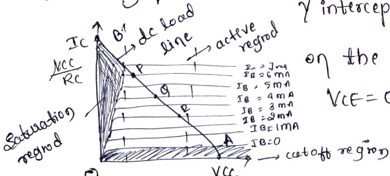
$V_{CE} = V_{CC}$  point A :  $I_C = 0$
