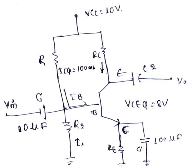
Determine the levels of  $I_{CQ}$  &  $V_{CEQ}$  for the voltage divider configuration using exact and approximation techniques.
