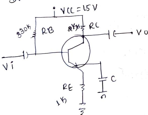
$$\begin{aligned} I_B &= \frac{V_{CC} - V_{BE}}{R_B + B R_E} \\ &= \frac{15 - 0.7}{330 \times 10^3 + 1 \times 10^3} \\ &= \frac{14.3}{430 \times 10^3} \\ I_B &= 33.2 \mu A \end{aligned}$$
