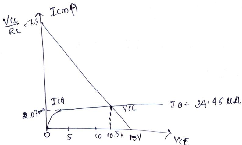
6) for the ckt shown below,  $\beta=100$ . calculate  $V_{CE}$  &  $I_C$
