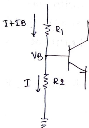
Let us consider the base ckt as shown in fig. The voltage across  $R_1$  is base Voltage  $V_{BE}$  applying voltage divider rule we get
