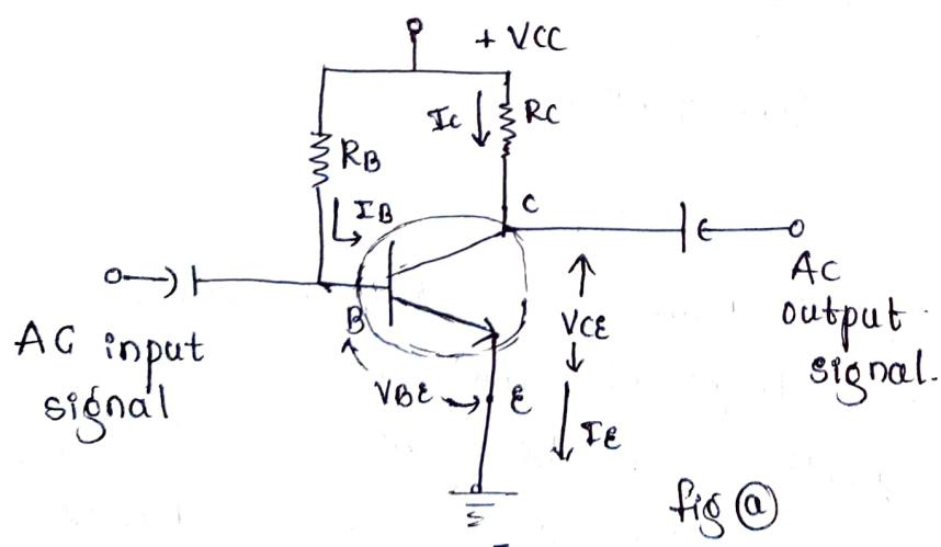
fixed bias ckt is shown in fig @ it is the simplest DC bias configuration. for the DC analysis we can replace the capacitor with an open ckt. The dc equivalent of fixed
