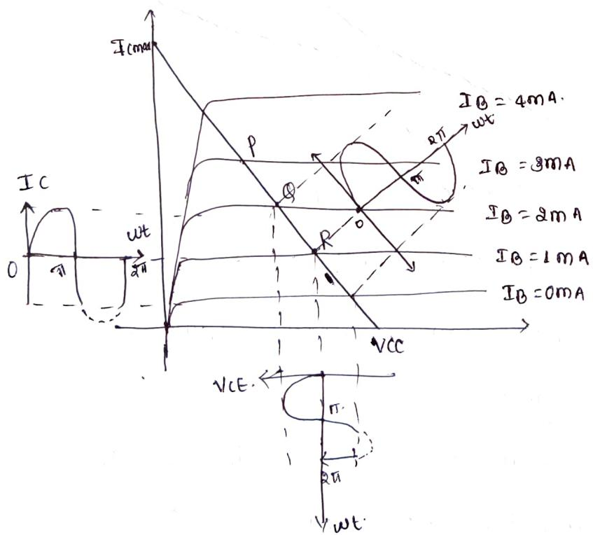
Biasing ckt is designed to fix a Q point at point 'R'. point R is very near to the cut off region shown in figure 3. the collector current is clipped at negative half cycle. Q<sub>0</sub> point R is not a suitable operating point.
