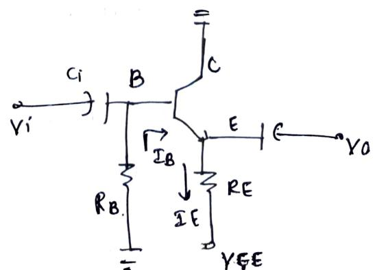
1) Determine the quiescent level of  $I_{CQ}$  and  $V_{CEQ}$ ,  $V_{CEQ}$  for the ckt shown in fig below. Repeat this problem using  $\beta$  of 135. Comment on the changes in the Q point.
