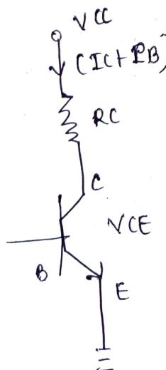
$$\begin{aligned} & (I_C + I_B)R_C + I_B R_B \\ & (B_1 I_B + I_B)R_C + I_B R_B \\ & \beta (I_B (B+1) + I_B R_B) \\ & R_B [(\beta + 1)R_C + R_B] \end{aligned}$$
