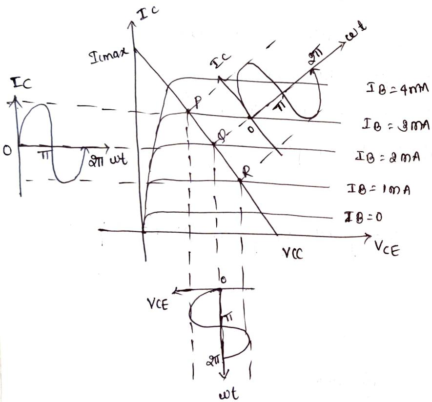
Biasing ckt is designed to fix the Q-point at point Q as shown in figure 6. the output signal is sinusoidal wave form without any distortion thus point Q is the best operating point
