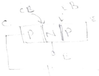
In order to operate transistor is the desired region we have to apply external dc voltages of current polarity and magnitude to the two junctions of the transistors. This is nothing but biasing of the transistor. Since dc voltages are used to bias the transistor, biasing is known as DC biasing of the transistor.
