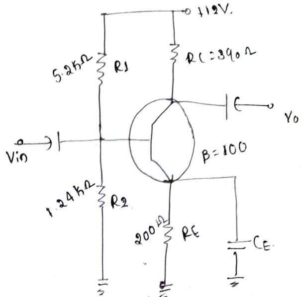
$$V_B = \frac{V_{CC}R_2}{R_1 + R_2}$$
