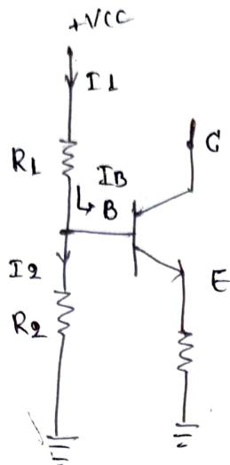
If we assume that current  $I_2$  is far greater than  $I_B$ , we can neglect  $I_B$  and  $I_1 = I_2$ .  $\therefore V_B = \frac{V_{CC}R_2}{R_1 + R_2}$
