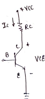
$$V_{CC} = \beta \cdot I_B R_C + V_{CE}$$
