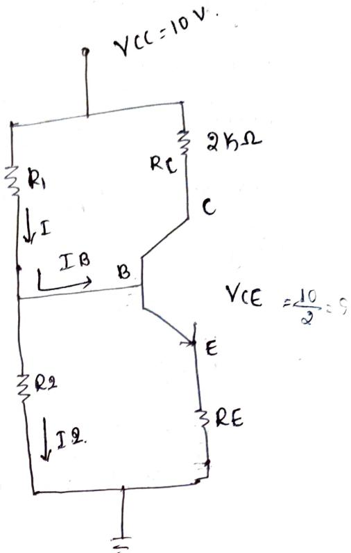
$$V_{CE} = I_C R_C - I_E R_B$$
