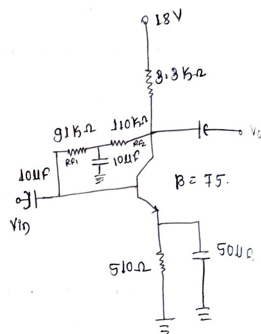
In DC ckt the capacitors are in open circuit.
