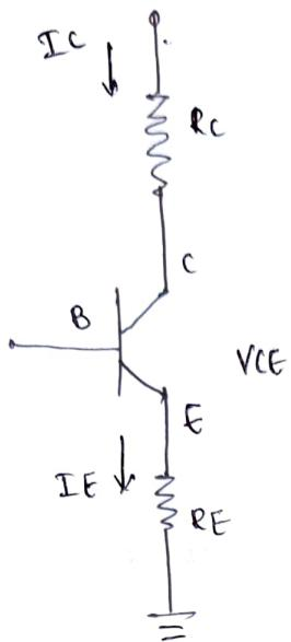
Let us consider collector ckt as shown in fig. Voltage across  $R_E$  can be obtained as.
