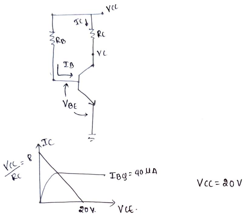
$$R_B = \frac{V_{CC} - V_{CE}}{I_B} = \frac{20 - 0.7}{40 \times 10^{-6}} = 0.4825 \times 10^6 = 482.5 \text{ k}\Omega$$
