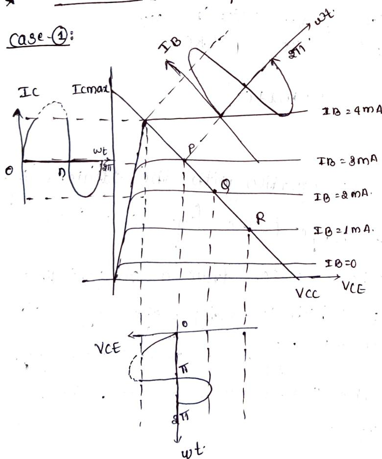
operating point of the transistor can be fixed at different points on the dc load line. Ex: P, Q, R.
