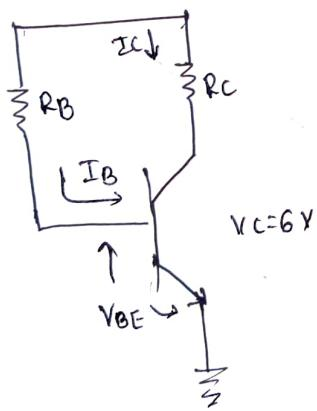
$$\begin{aligned} 1) \quad I_c &= \beta \times I_B \\ &= 80 \times 40 \times 10^{-6} \\ &= 3.2 \times 10^{-3} \text{ A} \\ &= 3.2 \text{ mA} \end{aligned}$$
