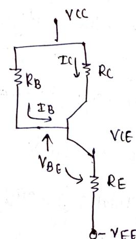
$$I_B = \frac{V_{CC} - V_{BE} - V_{GE}}{R_B + (1+\beta)R_E}$$
