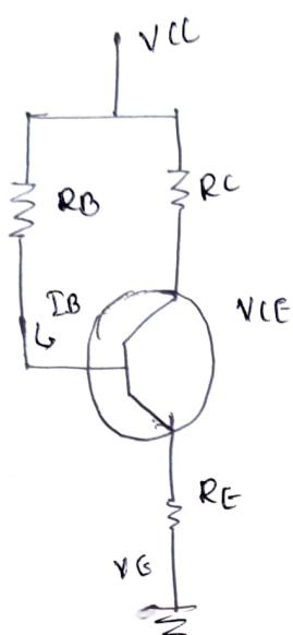
To improve the stability of the biasing ckt over the fixed bias ckt, the emitter resistance  $R_E$  is connected in bias ckt. Such biasing ckt is known as emitter bias ckt or self bias ckt.
