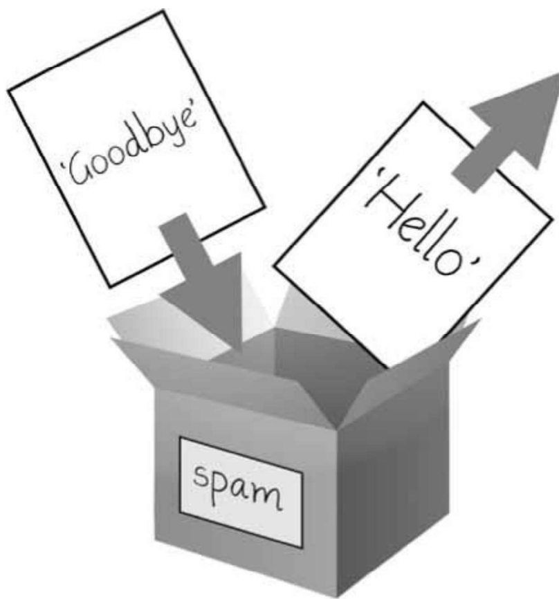
Figure 1-2: When a new value is assigned to a variable, the old one is forgotten.
