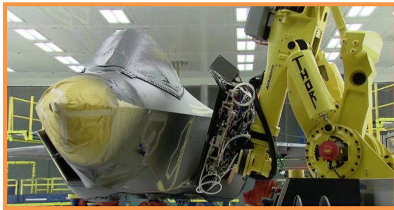
Figure13.1 Assembling of Aircraft Done by Robot
