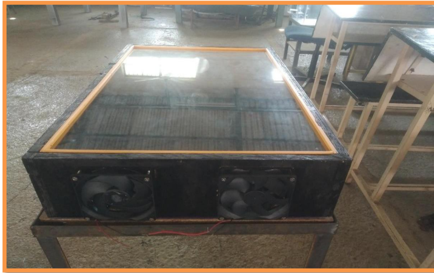
Figure 1.2 Solar Air collector
